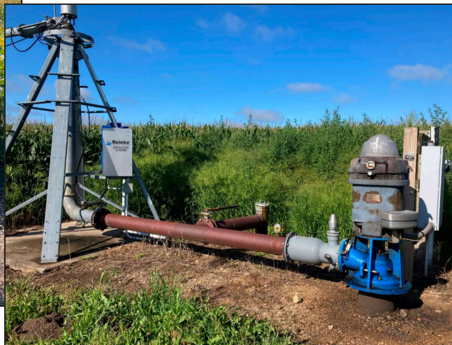
These photos illustrate a center pivot irrigation used to chemigate fertilizer only. When chemigating fertilizer only, operators are required to have one anti-pollution device.
