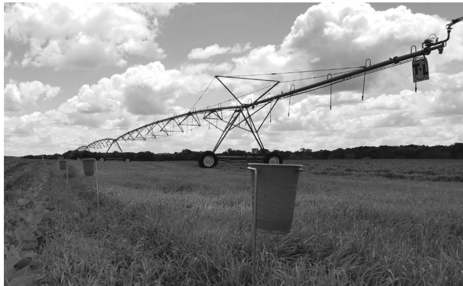
A uniformity test, also known as a "catch can test," is conducted by placing cups (catch cans) on stands 10 feet apart in a parallel line down the length of the pivot, then running the irrigator long enough to sprinkle at least 6 tenths over the cups.
