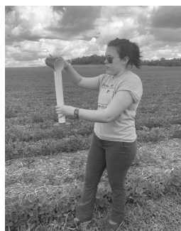
Tessa Zee, SWCD Conservation Planner, pours the collected water from the cup into a graduated cylinder and records the data.
