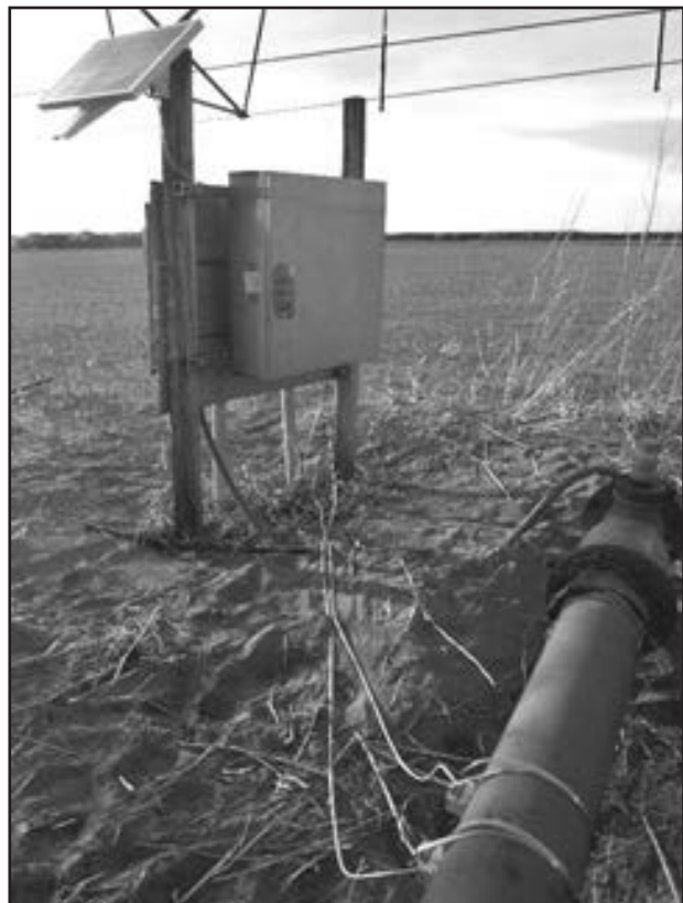
Parts of the flow meter system from upper left to lower right: solar panel, control box, two "clamp on" meters.
